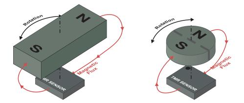
The sensor element free layers will align with the external field. As the applied field changes direction, the angle between the free layer and the pinned layer changes, changing the resistance of TMR elements, which changes the device output voltages.
